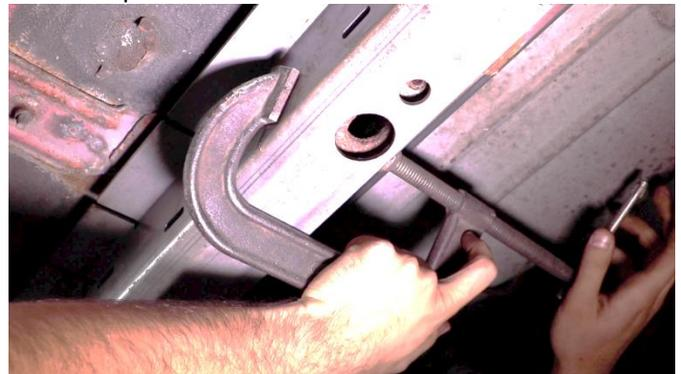
With another jack, press against the part at the bend point, ensuring the steel conforms to the shape of the rail.
