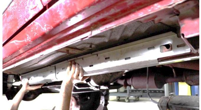
With the help of a friend or a jack, hold the part into place and begin c-clamping it to the rail, away from the bend point.
