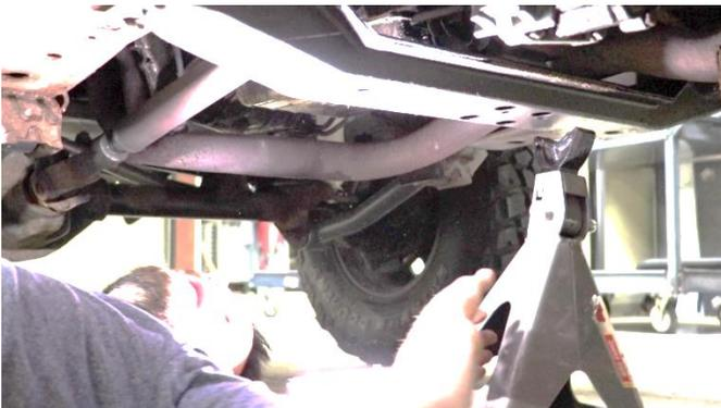
Prepare your weld zone by scoring or grinding away any rust and debris.
